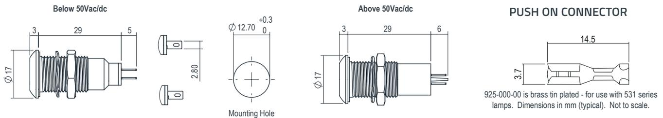
925-000-00 is brass tin plated - for use with 531 series lamps. Dimensions in mm (typical). Not to scale.
